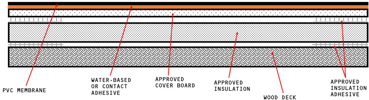
**APPROVED COVER BOARD:** DENS DECK, DENS DECK PRIME OR SECUROCK GLASS-MAT, MINIMUM 1/4" THICKNESS.
